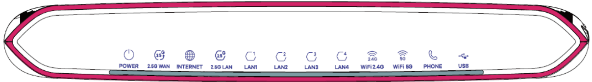
Figure 10 LED Indicators (EX5501-B0)
