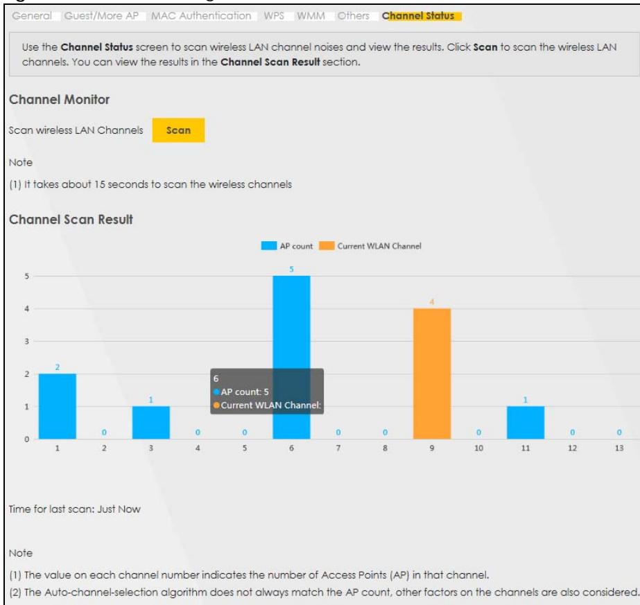
Figure 46 Network Setting > Wireless > Channel Status
